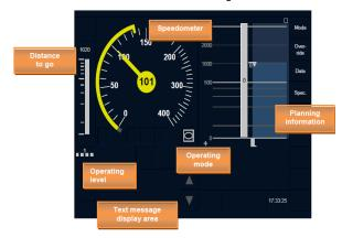
Typical Driver Machine Interface Display
