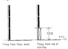
The use of tile fittings will be principally associated with the second category of tiling. Fittings will be required for internal and external corners and tiling perimeters. The dimensions of these fittings will depend on the distance between the faceline of the actual tiling and the nominal faceline of the wall. Particular consideration should be given to the internal corner.
